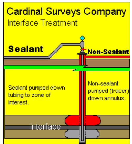
In this method, fluids are pumped from two different directions, and the depth at which they meet is the interface depth. In order to quantify the interface depth, a radioactive tracer can be injected with one of the treatment fluids so that the presence of the tracer in only one fluid accurately defines the interface location. The tracing and recording of the interface is known as an interface log.
